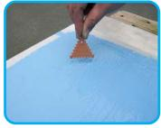
3. Use a wet film gauge to check the coating's wet film thickness (WFT) is at least 10 Mils.
